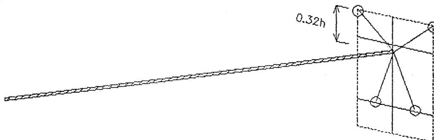
Note that other bridles hang with varying degrees of slack when the corners are drawn tight like this. Keep in mind that these figures are reported only to indicate a guideline for correct bridle proportioning since the problem is really about estimating the amount of catenary 'sag' which has to be built-in.
