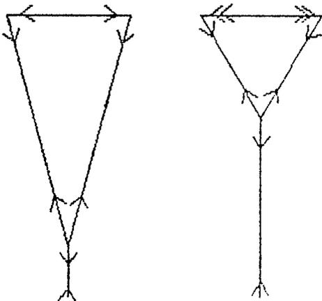
The force system involved is illustrated using the sign convention of structural engineers, where  $< >$  is compression and  $> <$  is tension.
