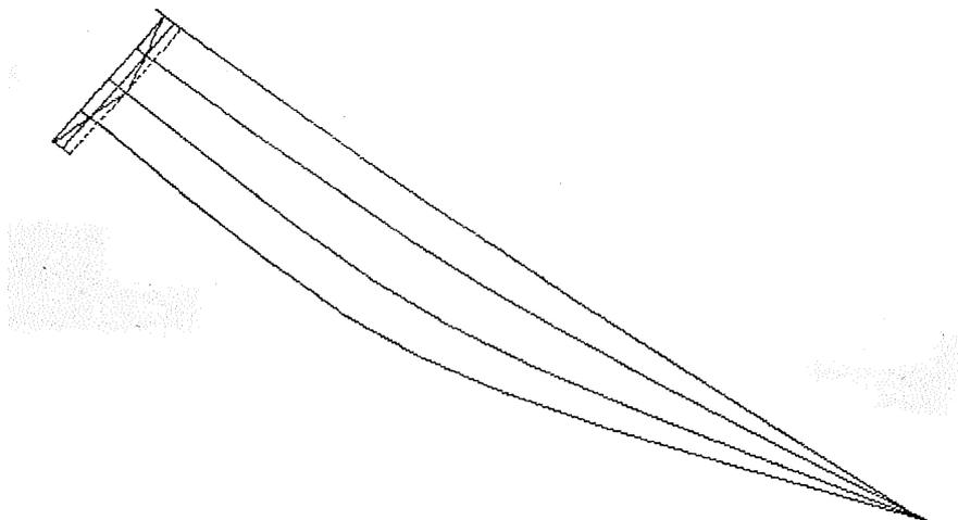
The difficulty in producing clear standard rules for location of the tow point in relation to the sail is that since each bridle set hangs in a slightly different catenary, then making any one set tight or fully tensioned will leave other sets either loose or overtightened.
